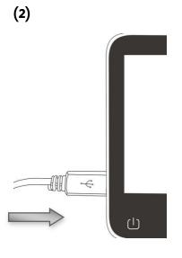
2、Turn on the APEX LOCATOR, insert other end of data transfer cable into APEX LOCATOR
