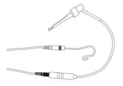
2. Connect file clip, measuring file and lip hook as shown in left picture.
