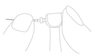
Installing the file: Insert the file and turn the file, make sure that file is inserted.
