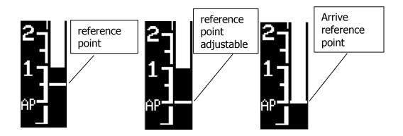
The position of the reference point is automatically setting with the APEX LOCATOR, and the cursor is displayed on the E-CONNECT screen.
