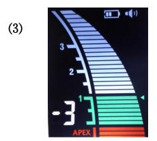
3. Observing APEX LOCATOR display, the root canal length strip will be all lighted, and a rapid beep sound will be generated at the same time, the 'APEX' sign will be flashed. That means the APEX LOCATOR is working normally.
