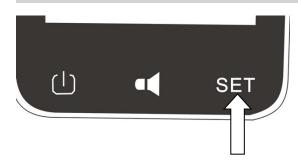
Press SET key , can setting the reference point , between  $0\sim1$ .
