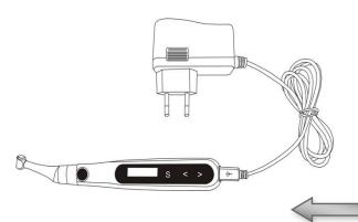
Connect the handle and adapter as shown.
